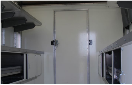
Full-height bulkhead door
