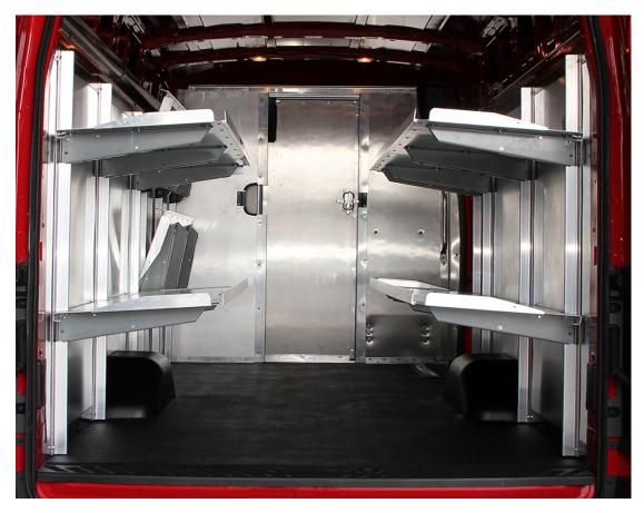
Utilimaster patented fold-up shelving maximizes cargo loading and flexibility. Includes aluminum side wall liner.
