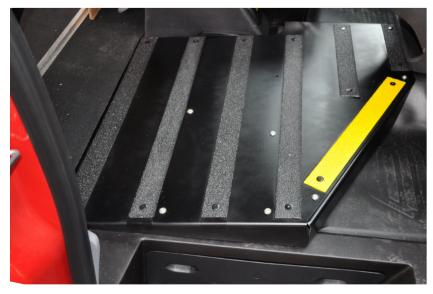
Flat floor kit with traction strips used when the passenger's seat has been removed.
