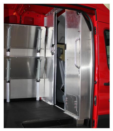
A heavy-duty bulkhead between the cab and cargo area provides additional security for the cargo and safety to the occupants.
