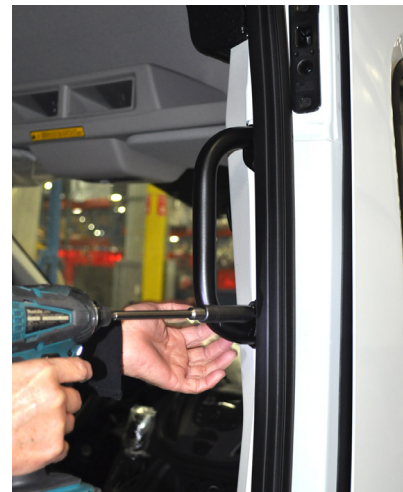
D-Ring at the LH side B-pillar and cargo grab handle on the RH side B-pillar
