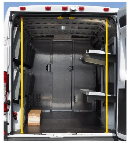
Ensure three-points of contact safety with a set of two floor-toceiling grab handles.
