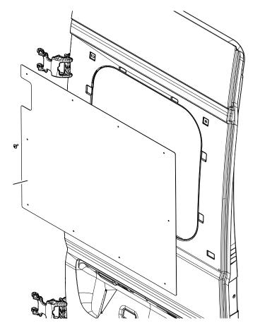
Increase cargo security by replacing the glass in the rear doors with permanent metal panels.
