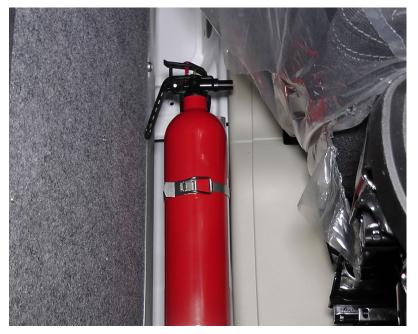
2.5# ABC disposable fire extinguisher with bracket to mount behind the driver's seat.
