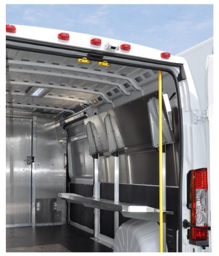
Utilimaster patented fold-up shelving maximizes cargo loading and usage.
