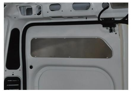
Two aluminum panels to close off the open cavities above the windows in the rear doors.
