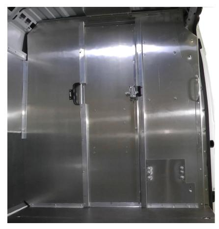
A bulkhead between the cab and cargo area provides additional security for the cargo and safety to the occupants.
