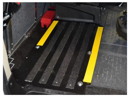
Flat floor kit with traction strips used when the passenger's seat has been removed.
