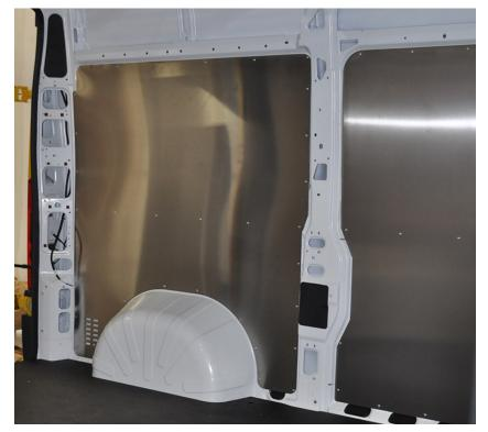
Durable aluminum panels to close off the open cavities in the sidewall.
