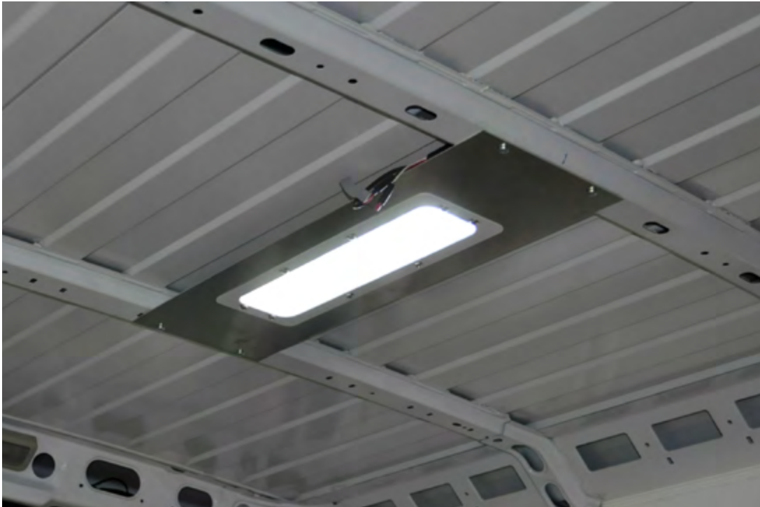
LED cargo light with motion sensor
