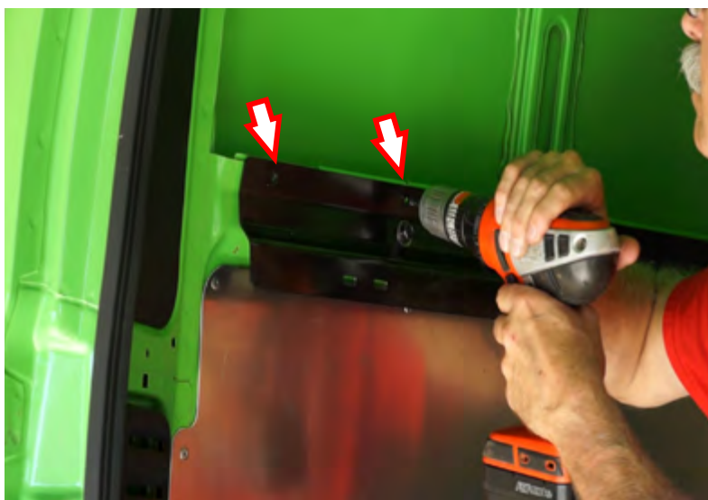
Drilled holes in sidewall and brace
