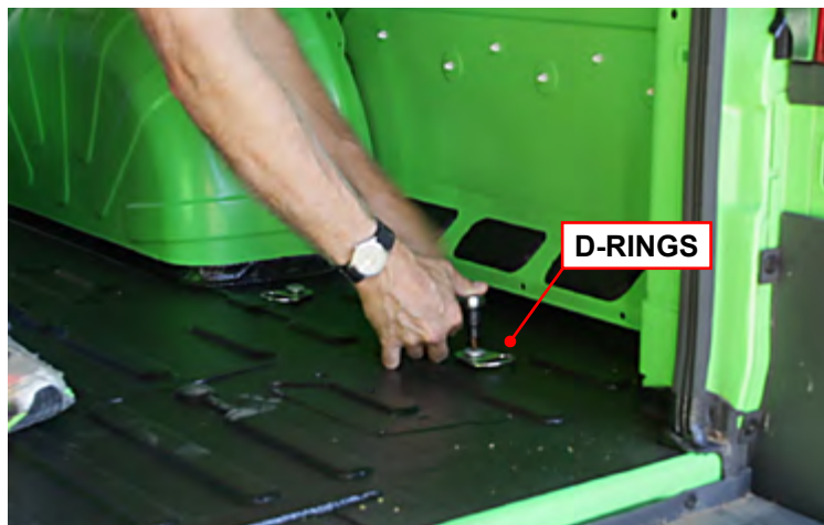
Remove cargo floor d-ring
