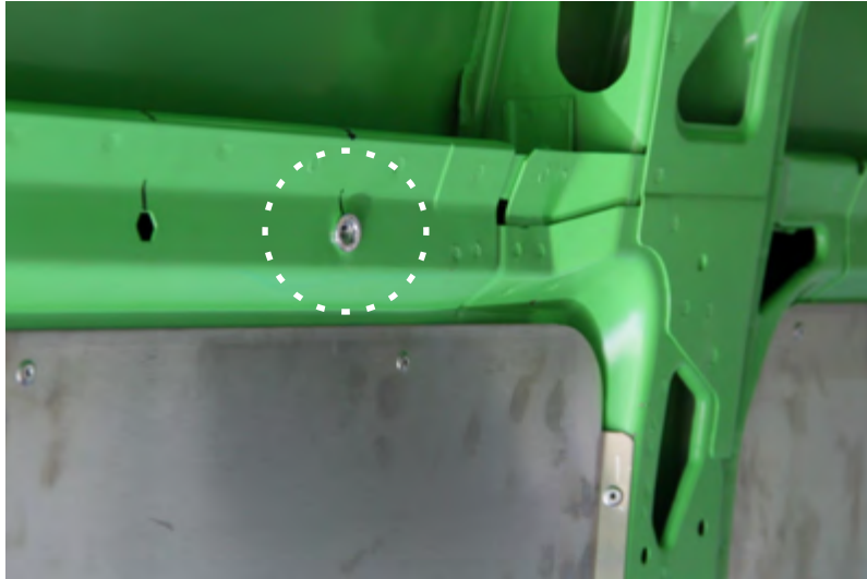
Hexsert installed in LH sidewall rib
