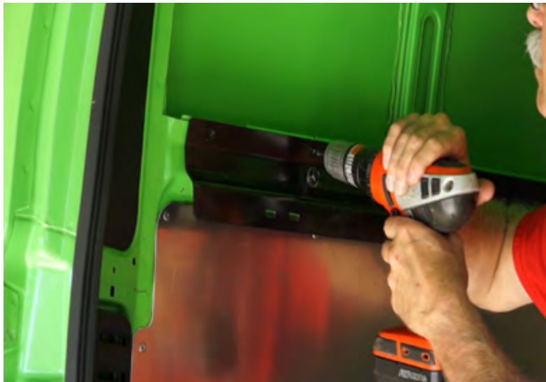
Drilled holes in sidewall and brace
