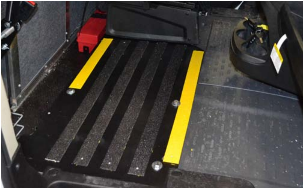
Cab floor overlay
