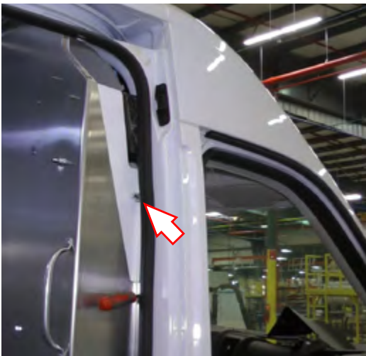
Fastener in upper B-pillar
