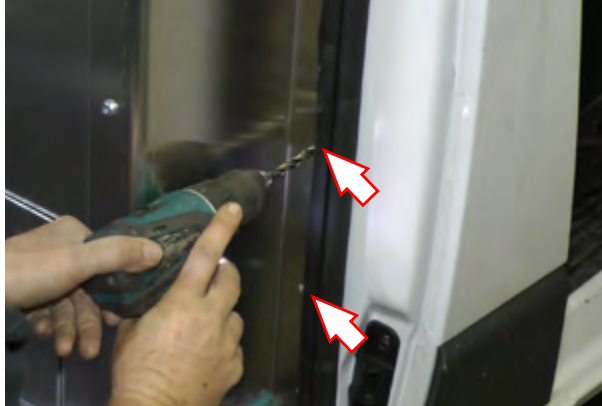
3/8" holes drilled in B-pillar
