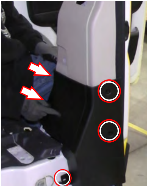
Lower B-pillar trim fasteners
