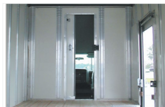
Full-height bulkhead door
