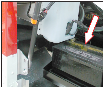
Battery Under the Hood
