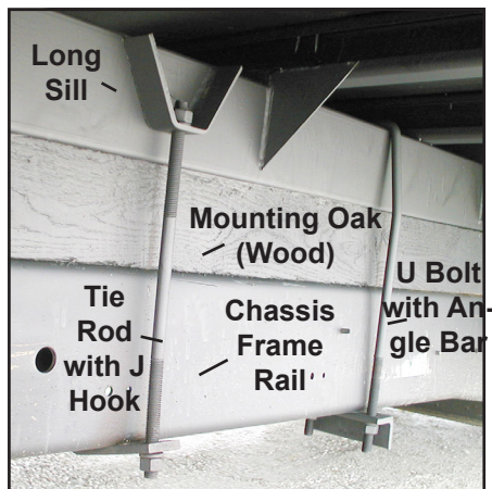
Truck Body Mounting Bolts
