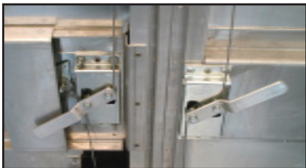
Lubricate Rear Swing Door Mechanisms
