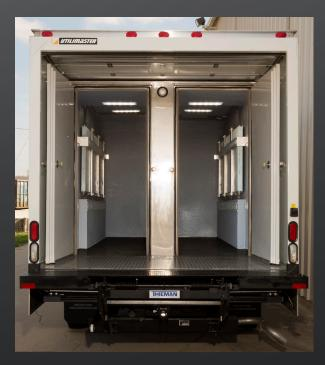
"Utilimaster designed and built a refrigerated truck to meet our exact needs with separate compartments for frozen goods, refrigerable goods and ambient goods."
