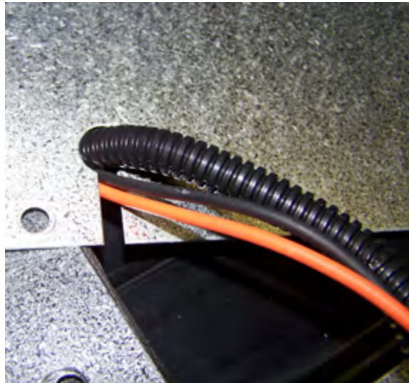
Place wires into convoluted tubing.
