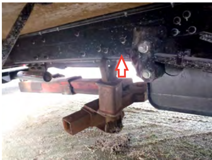
Lift the rear at the chassis frame rails (chains not yet installed).
