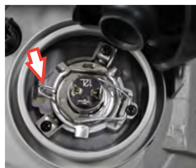
Spring securing headlight bulb
