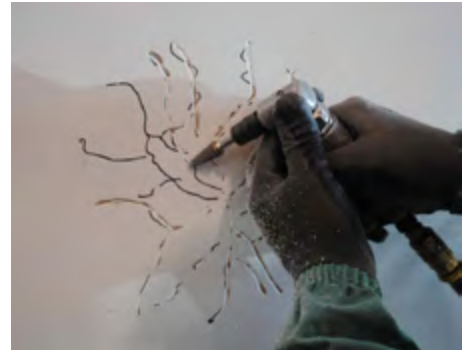
Use a die grinder to clean out gelcoat
