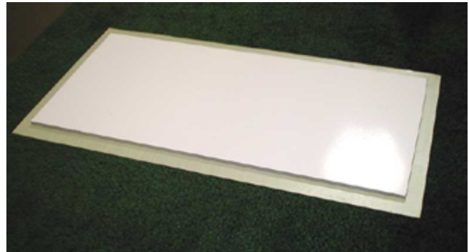
Inset panel set on self-adhesive patch panel
