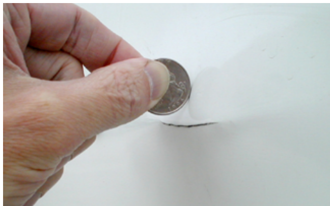
Tap across damaged area to test for delamination
