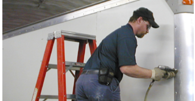
Removing panel fasteners
