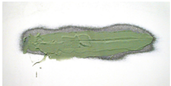
Body filler applied before final sanding and painting
