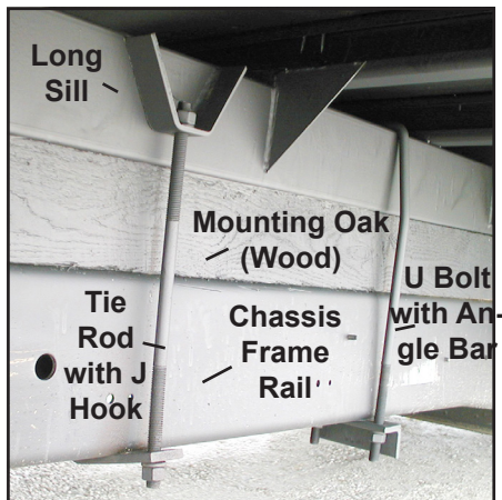
Truck Body Mounting Bolts
