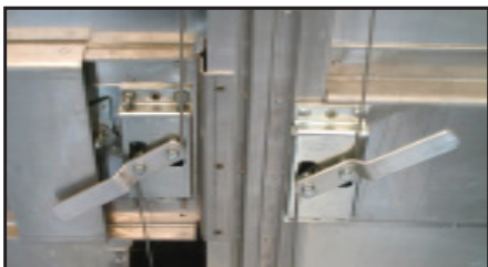
Lubricate Rear Swing Door Mechanisms
