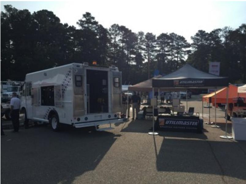
The 14' Utilimaster walk-in-van, designed, engineered, and manufactured specifically for Spartan Motors' customer Hawaiian Electric Company, is built on a Ford F-59 commercial chassis with a Kubota gas generator, Team Fenex air delivery system, and upfitted with EZ Stak interior cabinetry. This particular specialty service truck will be used to maintain and service the underground electrical infrastructure in Honolulu, Hawaii.
