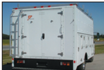
Rear Access Ladder and Racks
