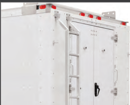
Rear Access Ladder
